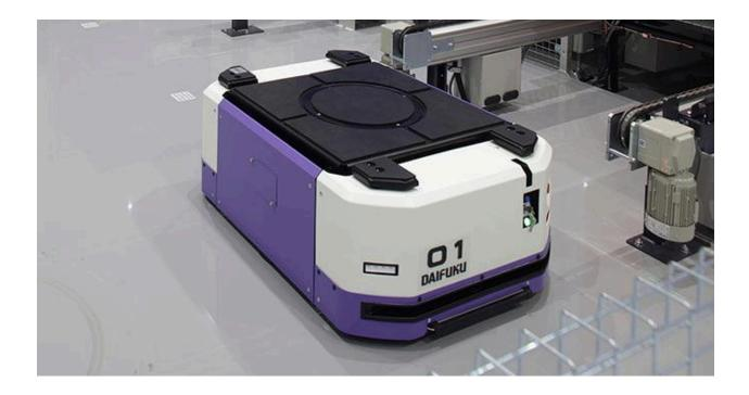
The <u>ASRS Vehicle System</u> by Daifuku optimizes warehouse operations through automated storage and retrieval, enhancing efficiency and accuracy. Designed for high-density storage, it utilizes advanced AGVs (Automated Guided Vehicles) to manage inventory swiftly, reducing labor costs and increasing throughput. Ideal for industries with high-volume storage needs.
