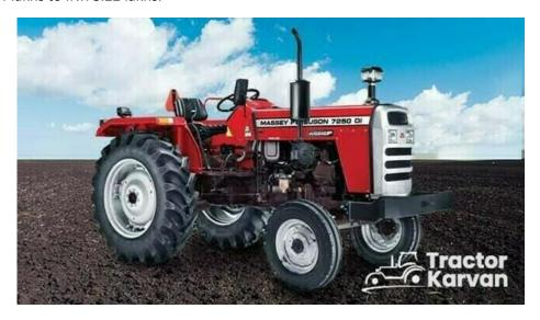
**Engine-** The Massey Ferguson 7250 tractor has 50 horsepower and three cylinders. It is driven by a SIMPSONS TIII A SJ327 engine, which guarantees that it emits less pollutants while completing any activity because it meets Trem III A emission requirements. The Massey 7250 engine has a capacity of 2700 cc.
